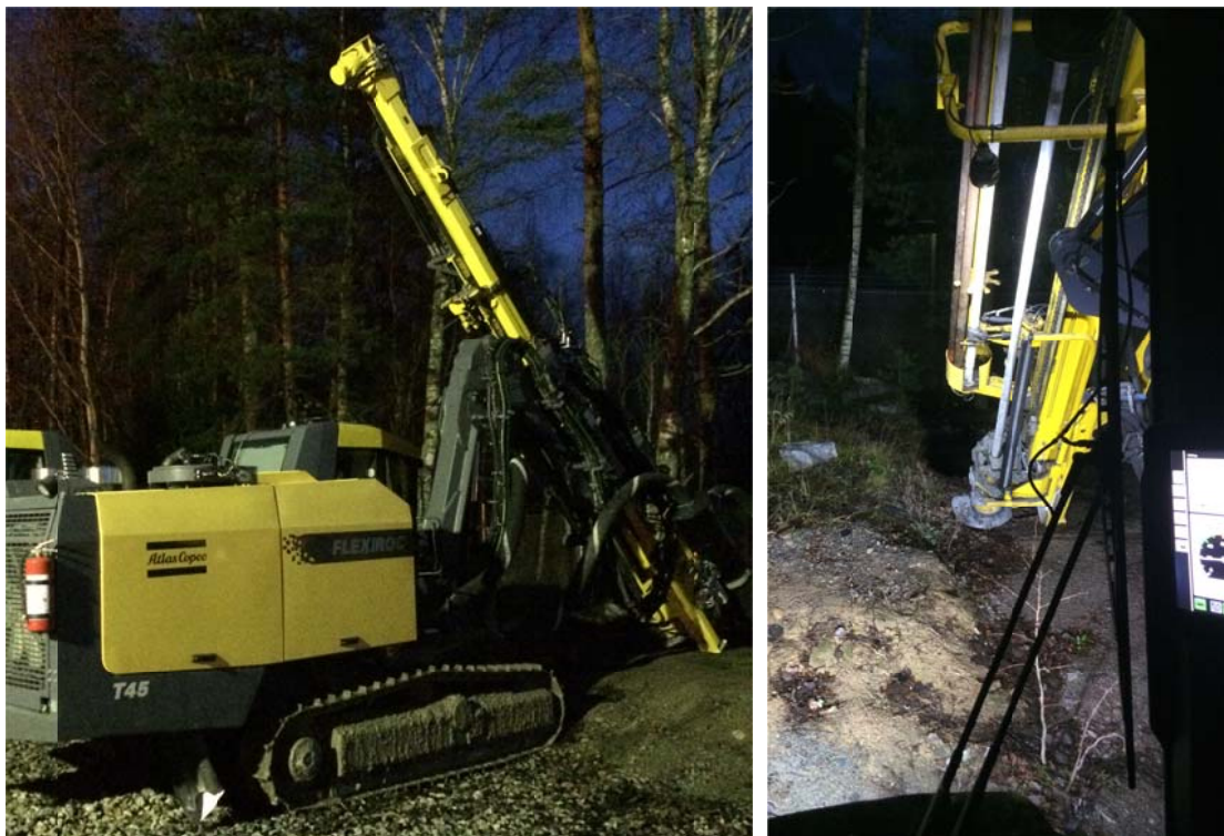
External and internal view of the Atlas Copco T45 drill used to drill test holes.
