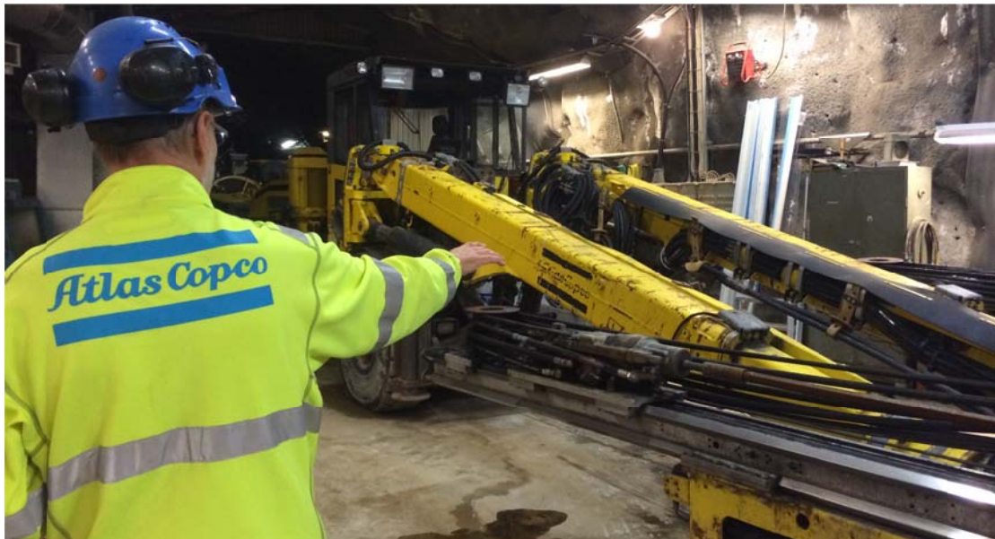
Lennart explaining out the features of a jumbo drill in the underground workshop.
