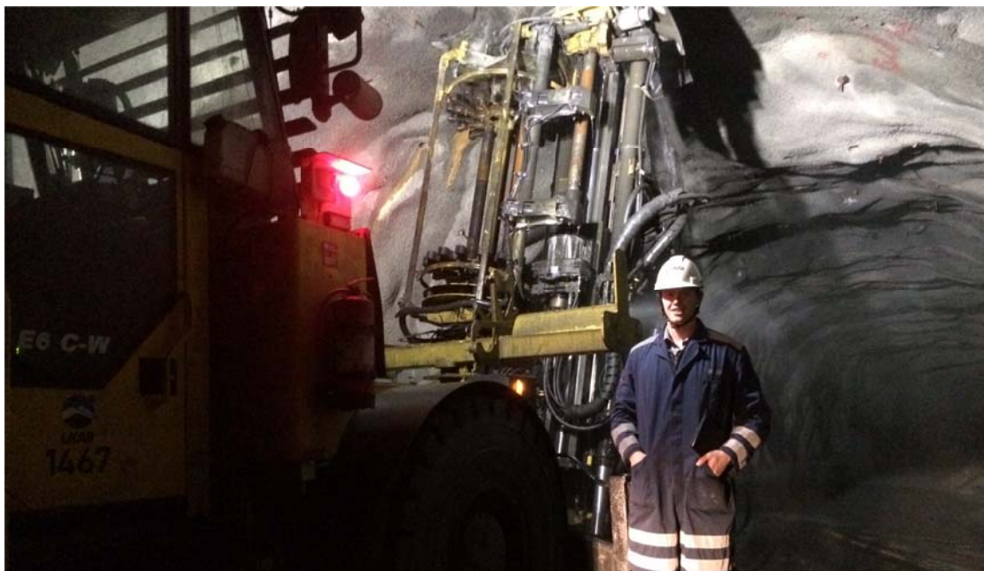
An autonomous Atlas Copco production drill rig in Malmberget.
