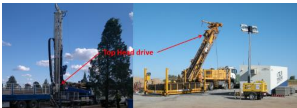
Figure A.2: Examples of top head drive rigs that may be encountered on a coal exploration or mine site (left is UDR 1200, right is a Bourne 750)
