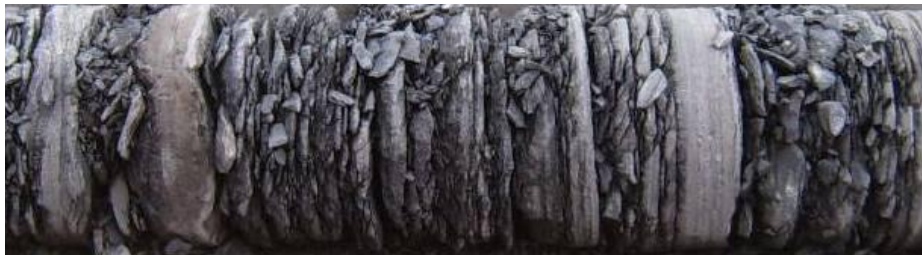
Figure 11.5: Example of Discing in Interlaminated Sandstone/Siltstone
