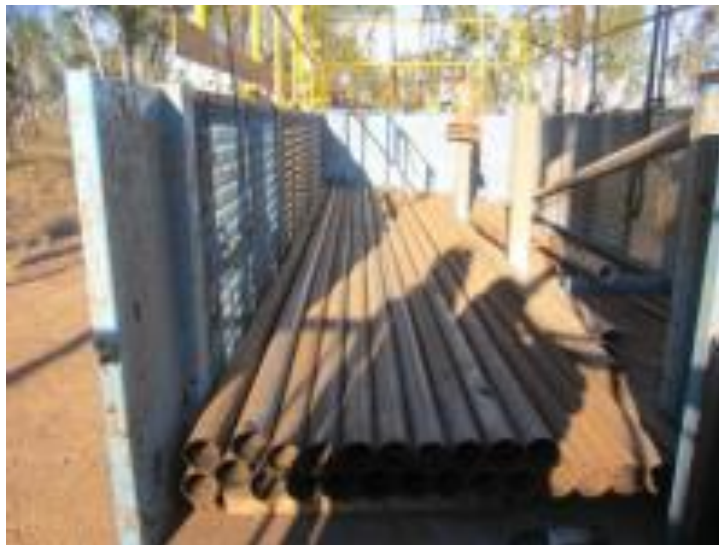
Figure A.5: Photograph A5: An example of a wire line HQ string of drill rods stored on a pod ready for Core drilling
