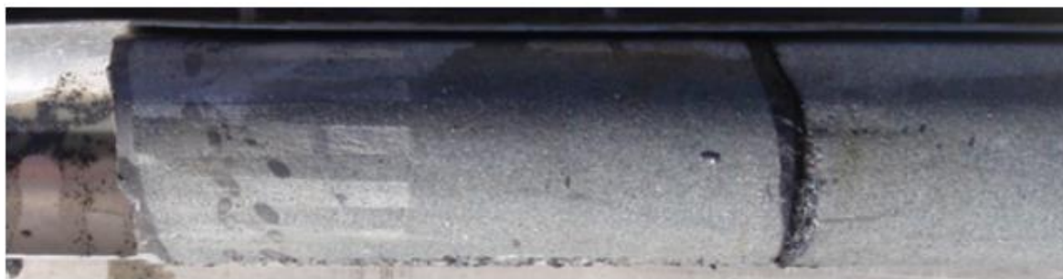
Figure 10.1: Catcher Marks at Top of Core Run Showing Recaptured Core
