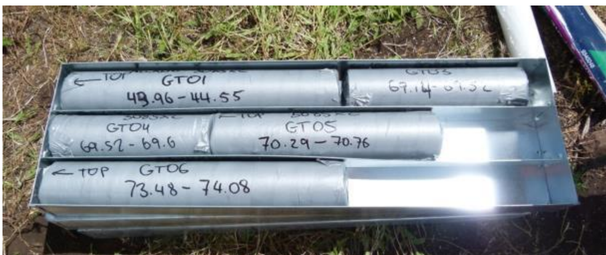
Figure 11.15: Geotechnical Samples in a Core Box
