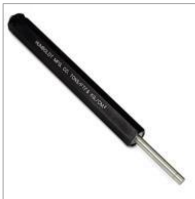
Figure 11.9: Example of a Pocket Soil Penetrometer (Humboldt) for Assessing Cohesive Soil Strength
