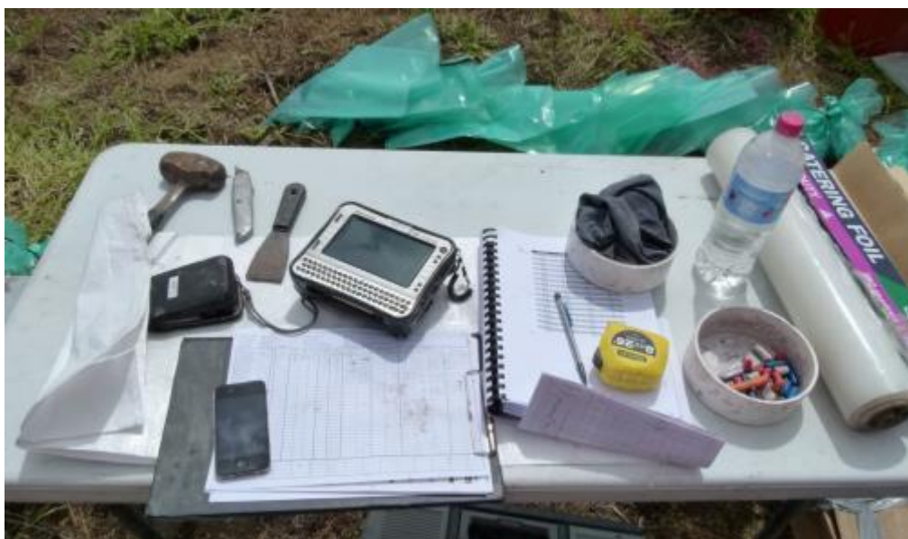
Figure 4.1: Equipment Prepared for Core Logging and Sampling
