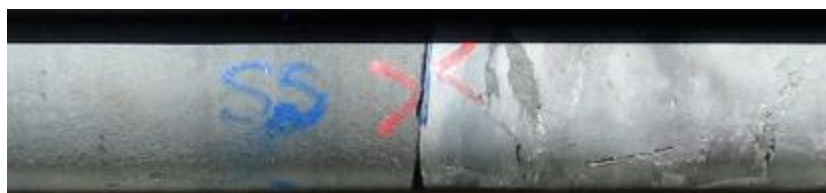
Figure 11.2: Example of a Broken Zone in a Claystone Unit
