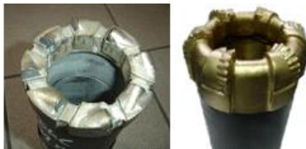
Figure A.11: An example of PCD/PDC coring bits
