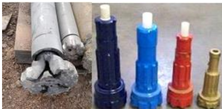
Figure A.9: Examples of hammer bits
