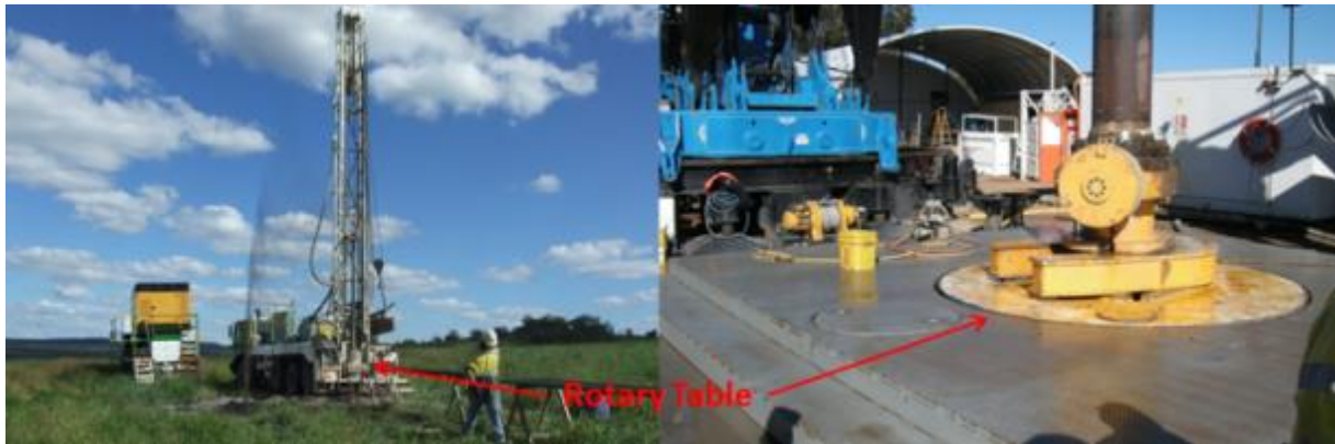
Figure A.1: Examples of table drive rigs that may be encountered on a coal exploration or mine sites (on the left is Bourne 1500 and the right is a shaft drill)
