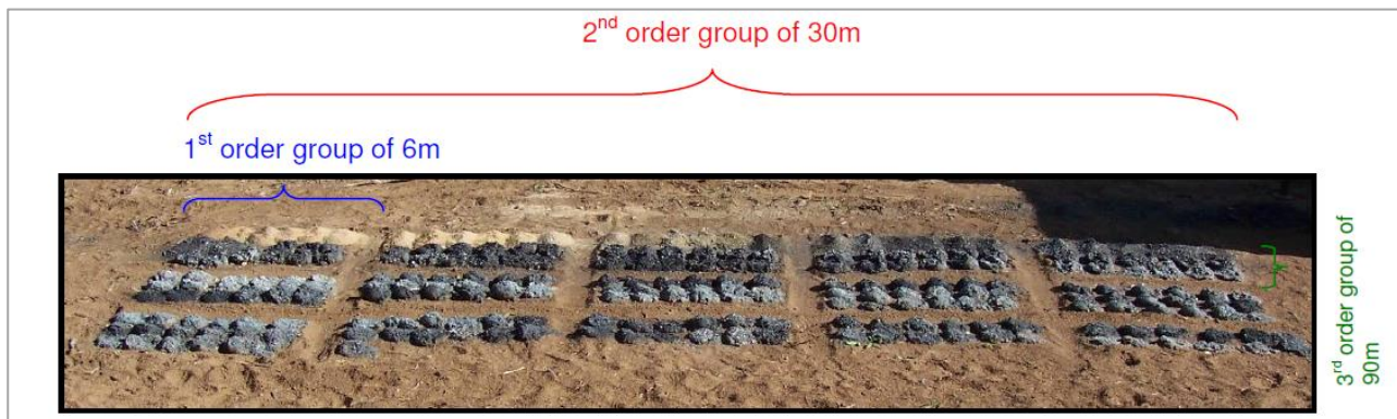
Figure 9.2: An Example of the Arrangement of Chip Samples
