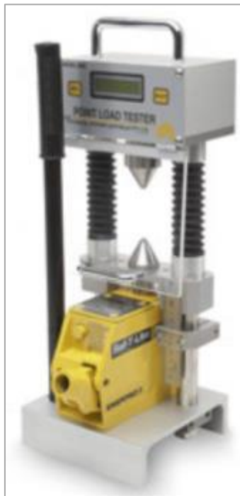
Figure 11.16: A Point Load Testing Machine
