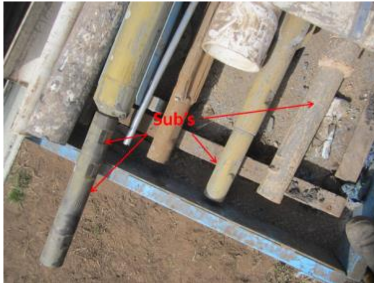
Figure A.13: Examples of drilling subs
