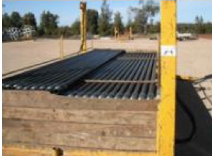
Figure A.4: An example of a typical string of drill rods stored on a pod ready for open/chip borehole drilling
