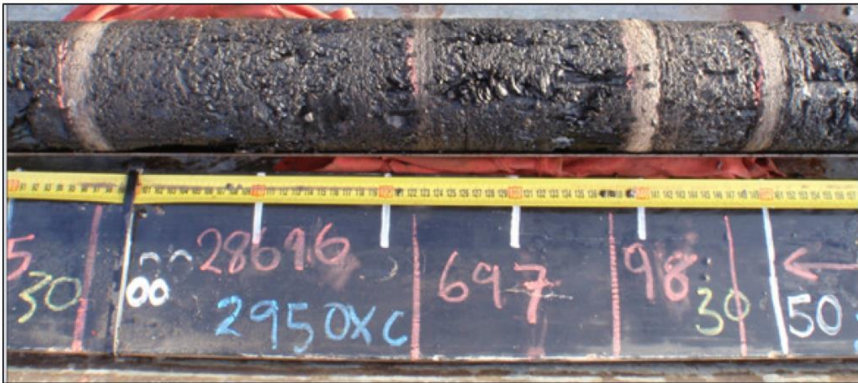
Figure 10.4: Example of a Core Photo on Logging Table
