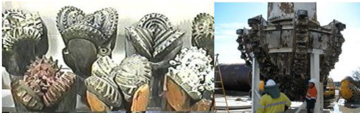
Figure A.6: Examples of rock roller bits
