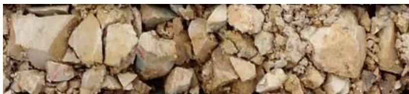
Figure 11.2: Example of a Broken Zone in a Claystone Unit
