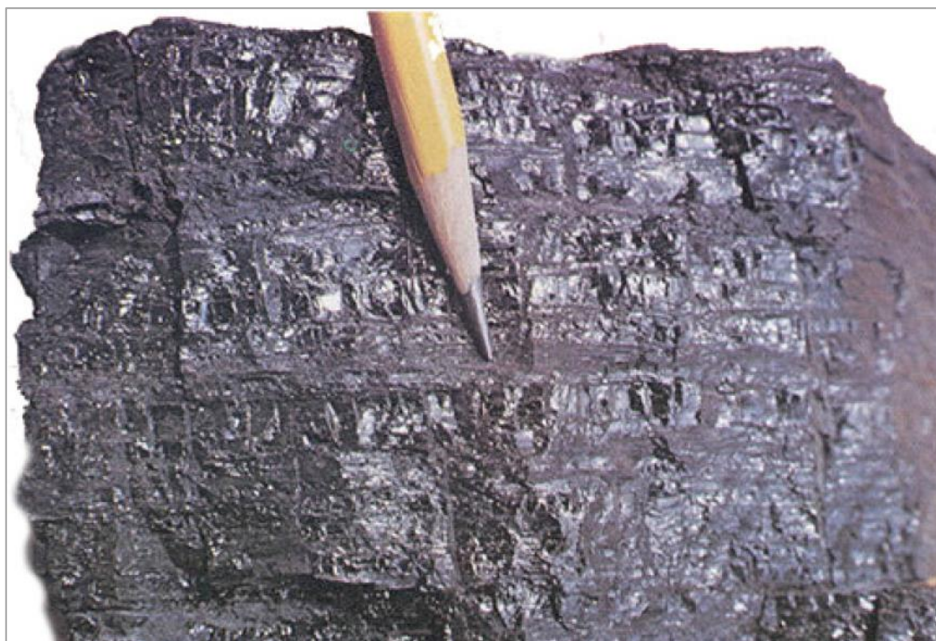
Figure 10.8: Example of Coal with 60 to 90% Bright Bands
