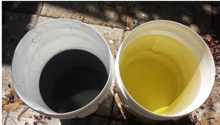
Separation of Graphite (L) & Graphene (R) at pH 2
