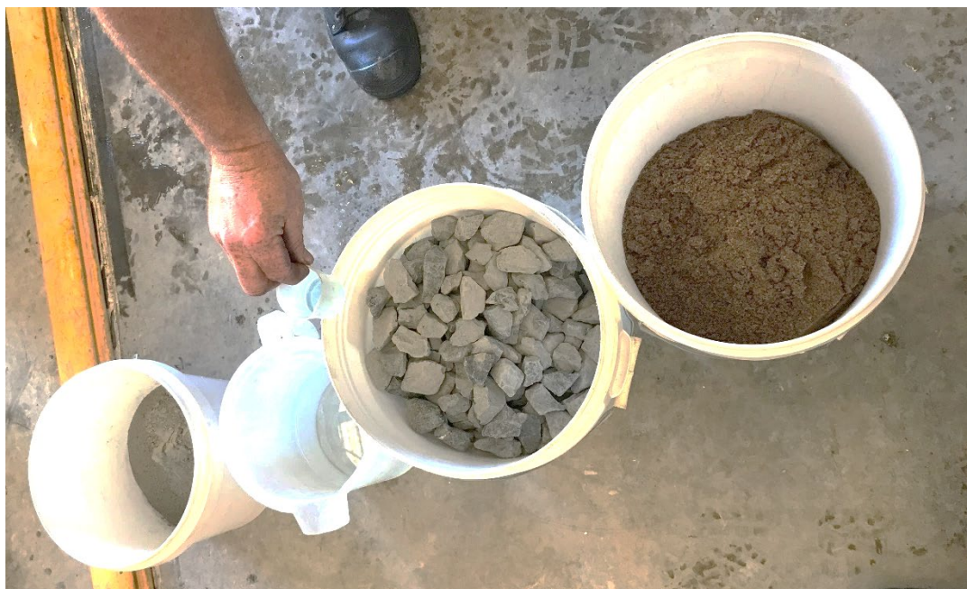
FIG 4 – Laboratory CRF samples being prepared for UCS testing. Additional aggregates were used but are not visible in this photograph.
