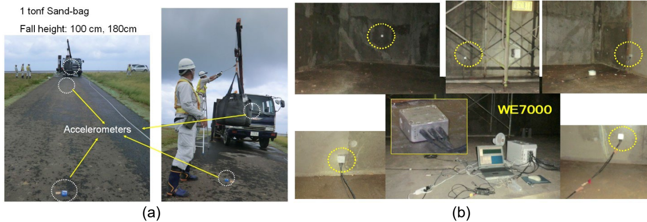
FIG 5 – Impact monitoring at a limestone construction site: (a) Impact location and position of sensors, and (b) recorded accelerations (from Aydan, 2017b).
