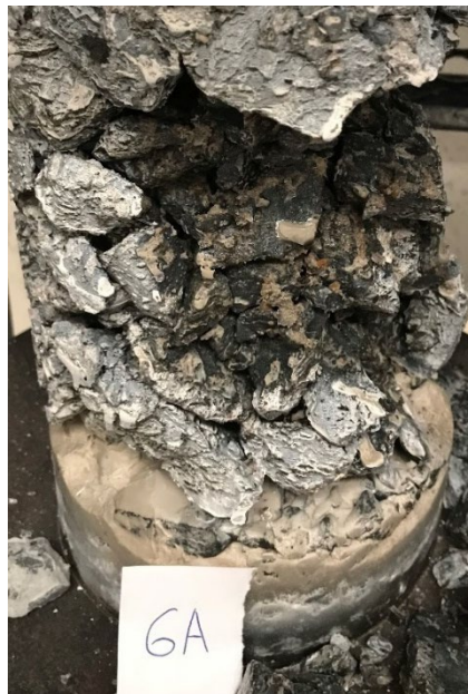
FIG 8 – Photograph of CRF cylinder showing clear segregation of the cement slurry from the aggregate. Note the colour change in the base of the cylinder, as well as the lack of slurry coating the large aggregate.
