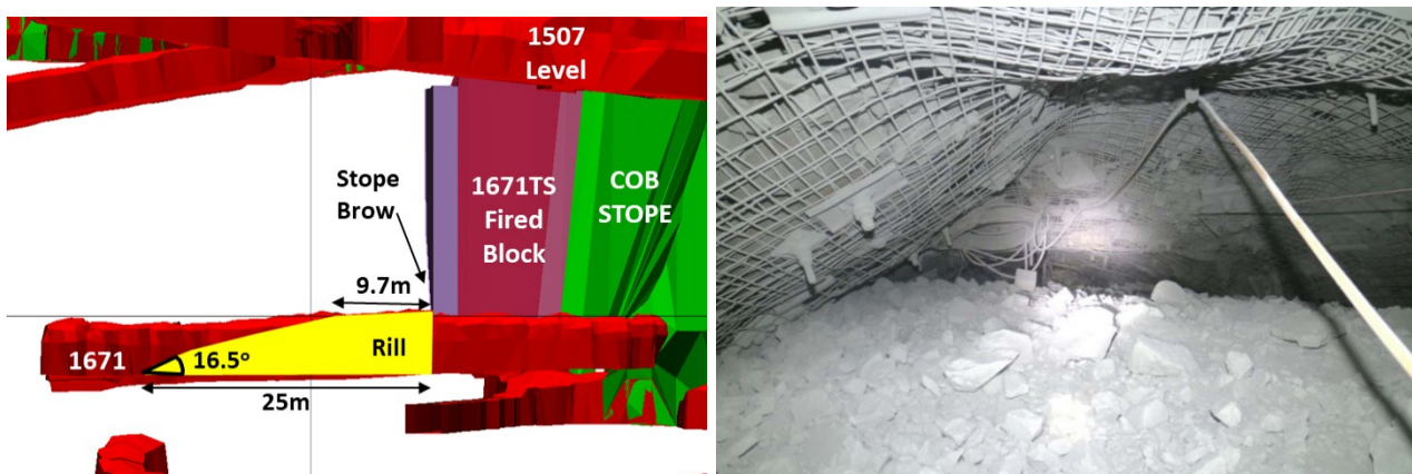
FIG 10 – (left) Cross-section looking west of the COB stope and 16 Level TSB#1. The material expelled by the blast is highlighted yellow. The first 10 m of the rill was tight filled to the backs, and the rest rilled at an angle of 17° to a total distance of 25 m from the designed stope brow. (right) View in 1671 drive looking north, taken from about 15 m from the TSB#1 brow. Fired material is packed to almost the backs of the drive.
