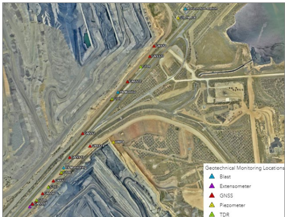
FIG 6 – Monitoring installed in the infrastructure corridor.
