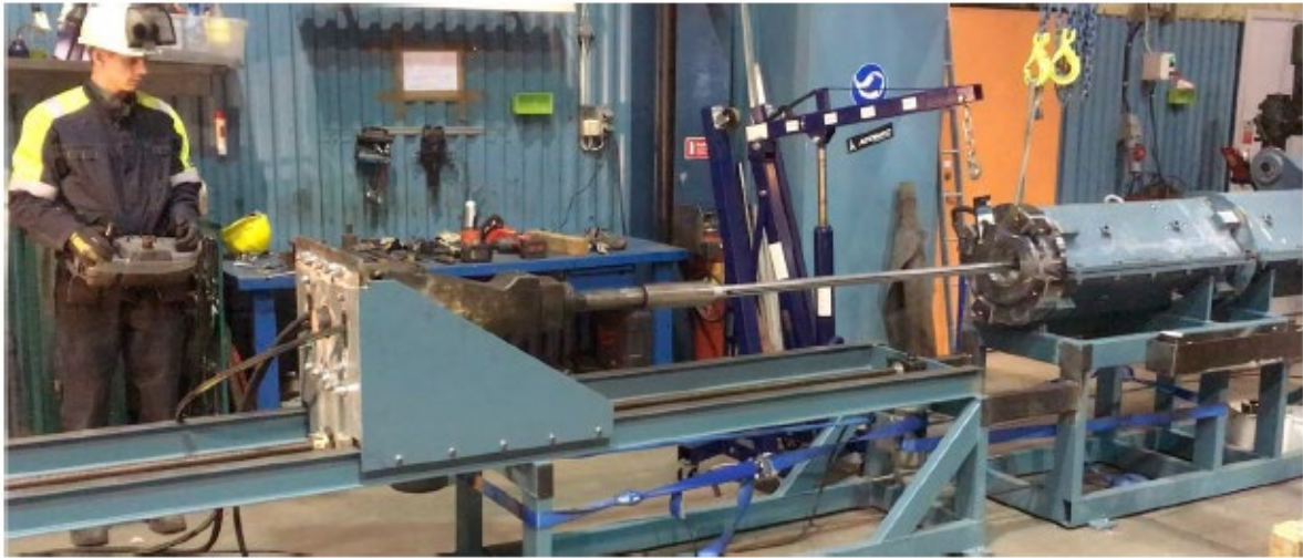
FIG 7 – Bolt installation rig.
