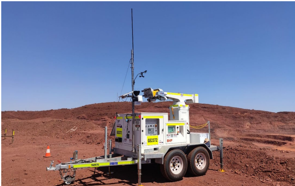
FIG 2 – WAIO Slope Radar monitoring system.
