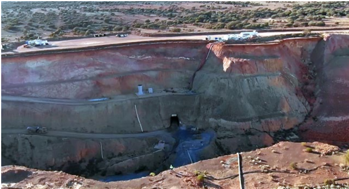
FIG 2 – Mine entrance portal in the existing Vivien Pit (courtesy of Ramelius Resources).
