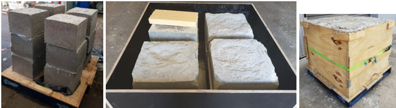
FIG 1 – Prepared samples. Left: without interface sample; Centre: with interface sample; and Right: example of the sample ready for drilling experiments.
