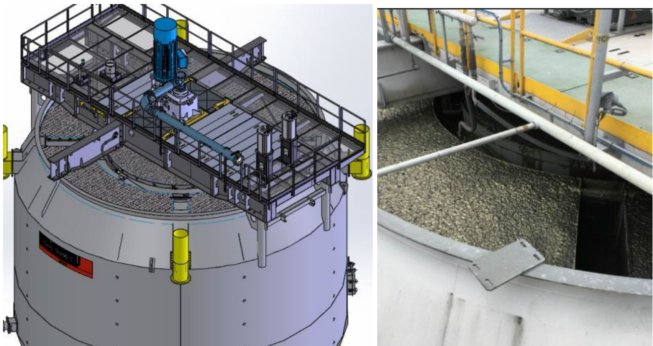
FIG 4 – TankCell e630 with a centre launder.
