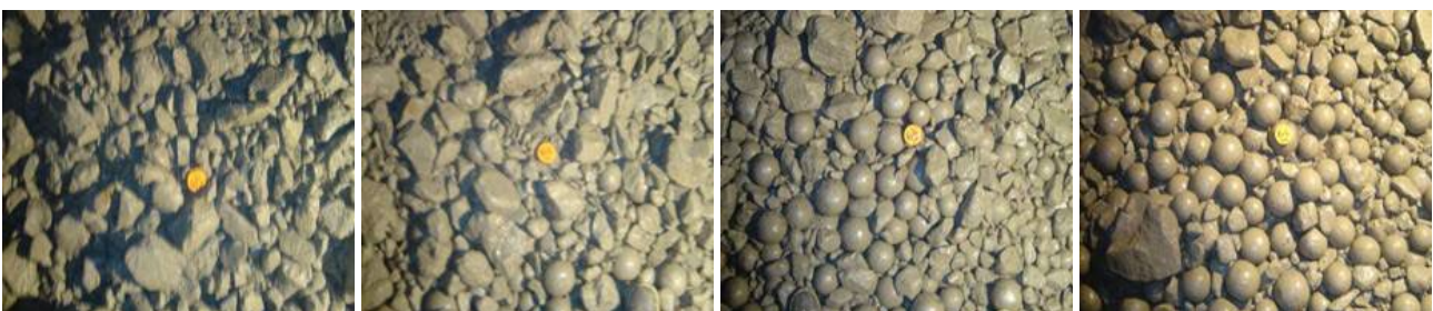
FIG 3 – Segregation from feed to discharge end of a 32 ft diameter, 16 ft long SAG mill (left: feed end; right: discharge end).
