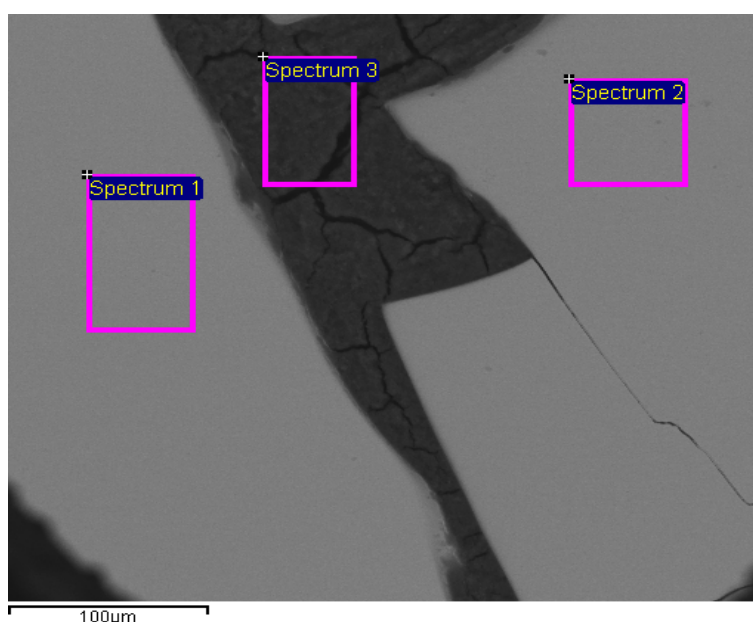
FIG 3 – BSE micrograph of the natural sperrylite electrode.
