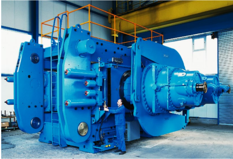
FIG 2 – Typical example of a state-of-the-art HPGR.
