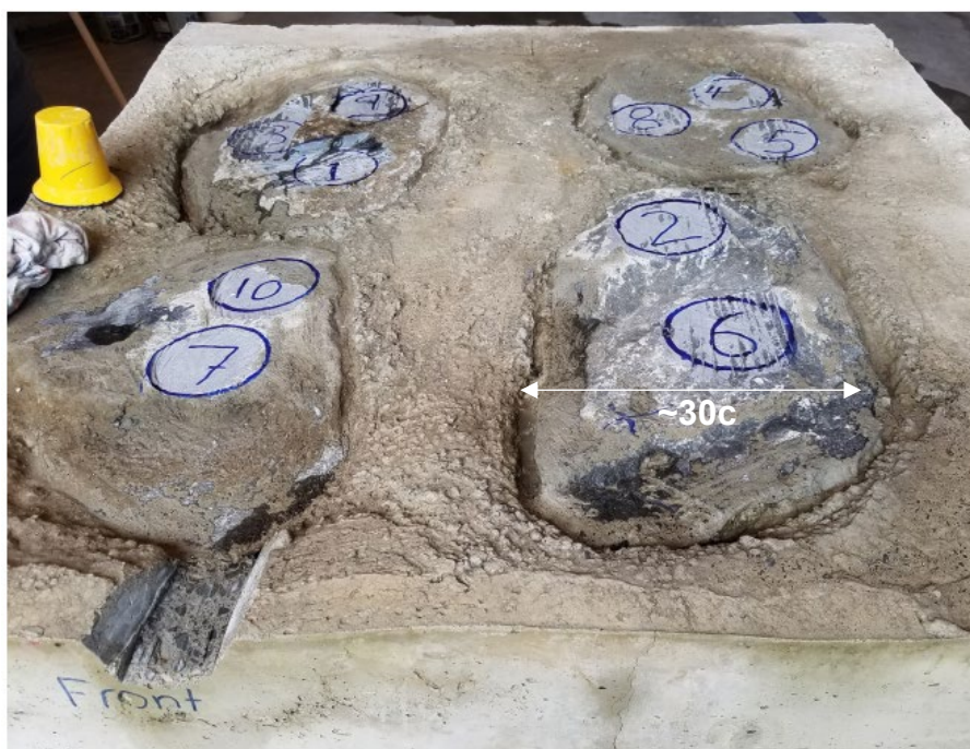
FIG 1 – Concrete block with four rock samples prepared for drilling.
