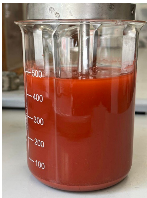
FIG 3 – Selective flocculation of silica using cationic flocculant when dispersant dosage of 300 Na-HMP/t \text{SiO}_2 is used for 1 wt per cent suspension containing 1:9 hematite and silica in 0.01 M KCl at pH 10.
