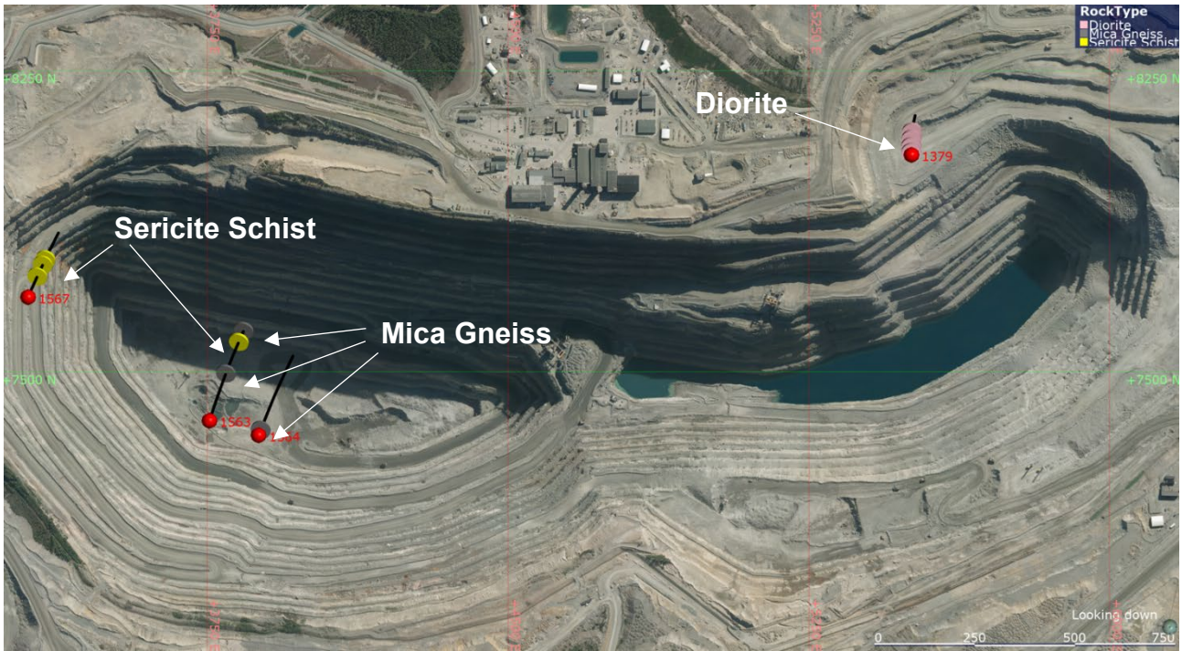
FIG 1 – Plan view of the Aitik open pit mine with the locations of the drill holes from which samples were retrieved. The disks are coloured according to the different rock types (red = Diorite, grey = Mica Gneiss, yellow = Sericite Schist) and illustrate the approximate depths of the samples.
