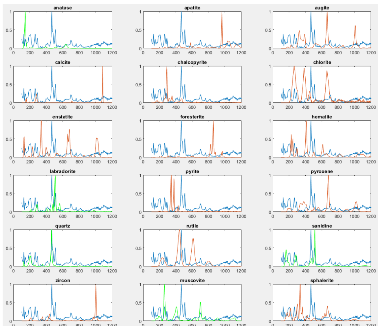
FIG 5 – Feature extraction from mixed Raman spectra: The blue line shows the mixed spectrum from a profile measurement. The green line shows a reference spectrum of a mineral found in the mixed spectrum. The red line shows a reference spectrum of a mineral that is not identifiable in the mixed spectrum.
