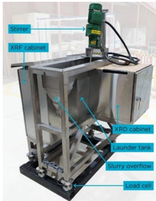
FIG 1 – Photograph of the MEA with the main components labelled. The system consists of X-ray instrument enclosures that are mounted to an 80 L launder tank. The analyser has a footprint of approximately 2 m 2 .
