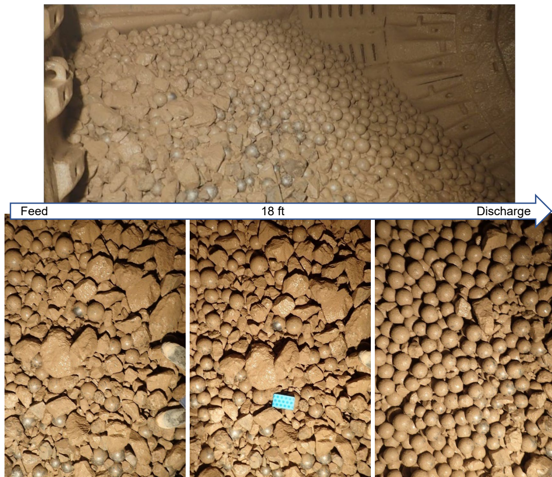
FIG 4 – SAG mill 21 per cent filling, 11 per cent balls.
