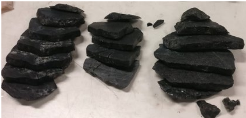
FIG 1 – Sliced large stones for preparation of small drill cores.
