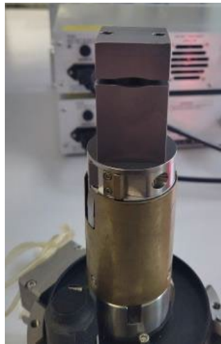
FIG 2 – Deben CT5000 TEC unit at GTK used for compression tests. The Brazilian loading test apparatus is on top of the loading cell.
