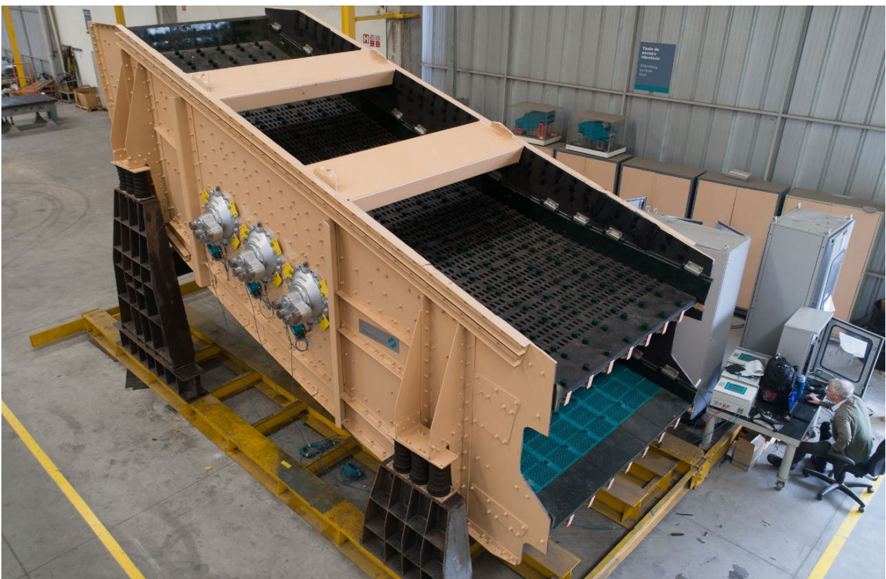
FIG 8 – SED2564 electronic synchronisation testing in Tabaute workshop.
