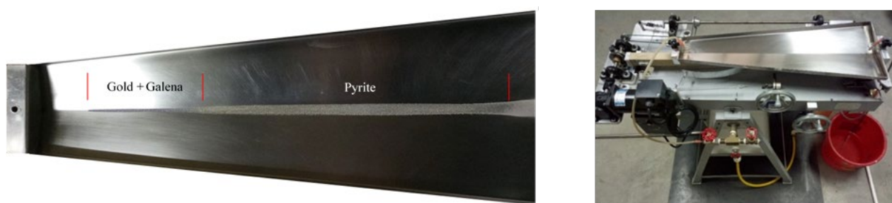
FIG 2 – Photographs showing the separation of a sulfide gold ore (left) by superpanner (right) Gold, galena, pyrite and silicate fraction were well separated.
