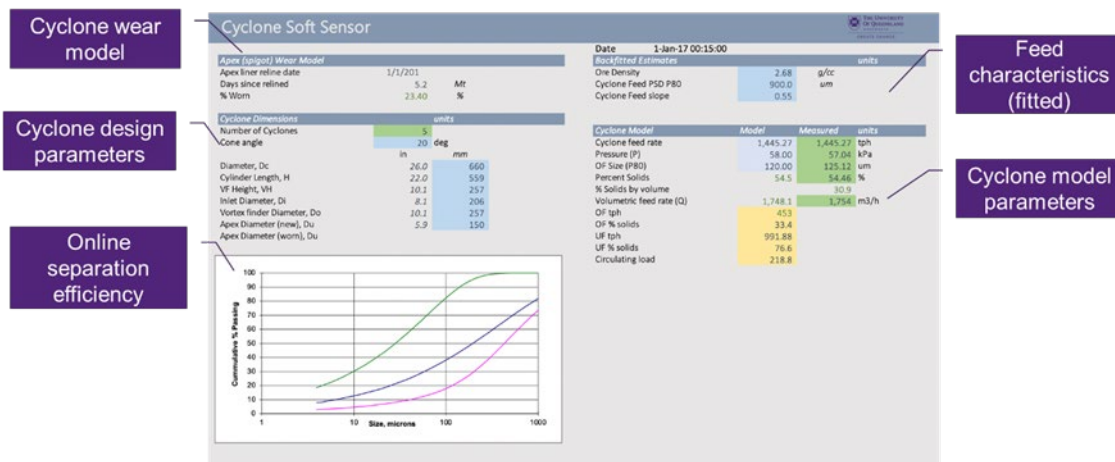
FIG 3 – Dashboard of the JKMRC hydrocyclone performance soft sensor prototype. Online inference (yellow cells) of the feed properties, as well as the water and solids split, are provided using existing instrumentation (green cells).
