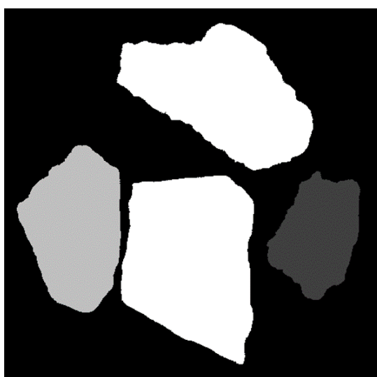
FIG 3 – A cross-section of segmented 3D XMT image where each particle is segmented and assigned a unique label number.
