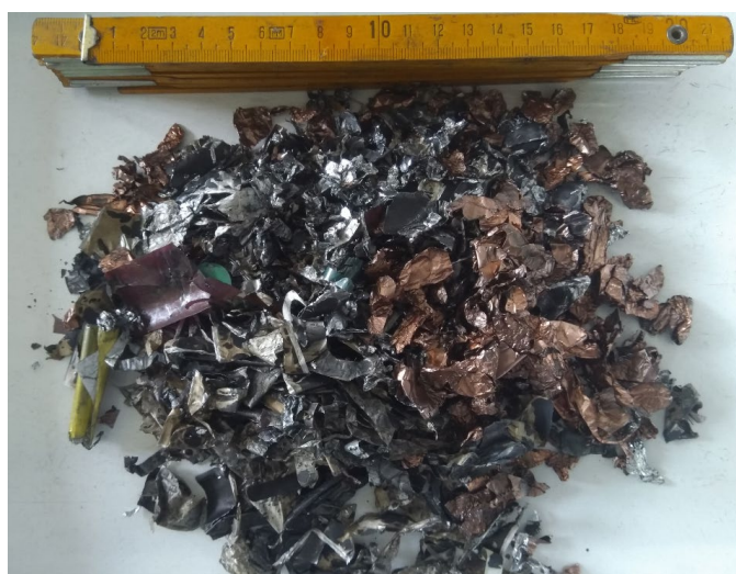
FIG 3 – Electrode foil mixture after first Zig-Zag-air classification.
