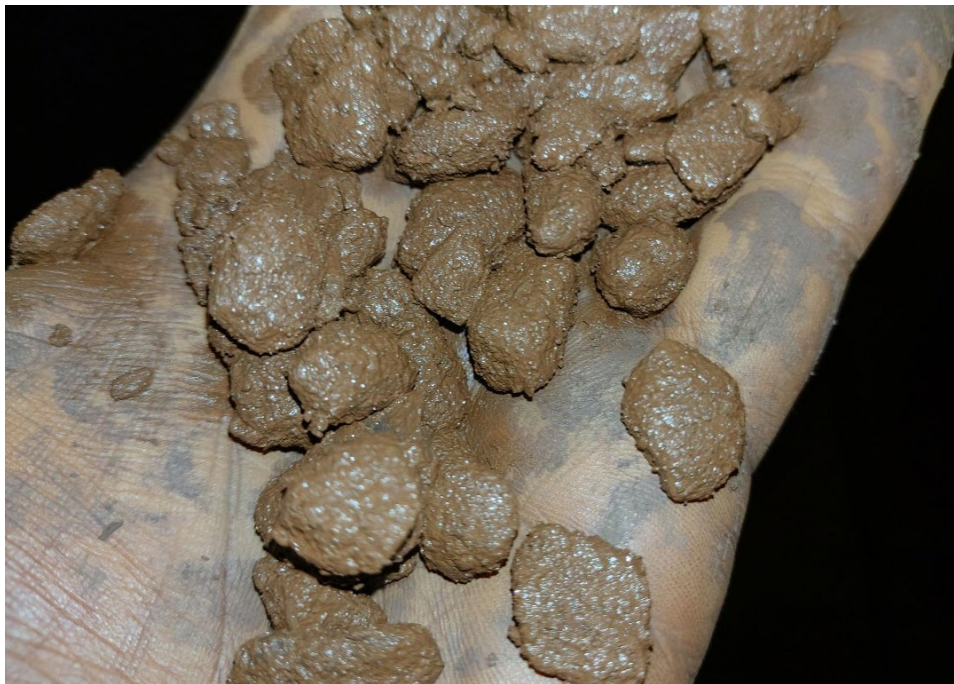
FIG 10 – Agglomerated fines obtained from the undersize of the screen whilst operating with high surface moisture content.
