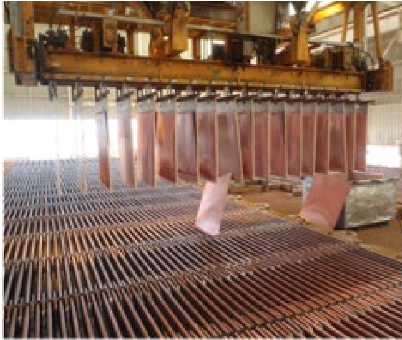
FIG 2 – Example of copper cathode pre-strip in EW.
