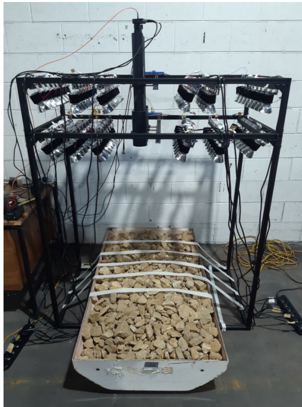
FIG 1 – The full-scale fluorine-mineral sensor prototype, showing the scale of the system, the LED arrays, and the detection optics (centre).
