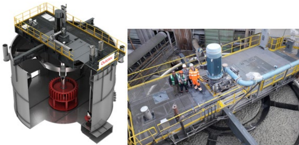
FIG 2 – Schematic image of TankCell e630 and the flotation cell at BVC concentrator (Grau et al , 2018).
