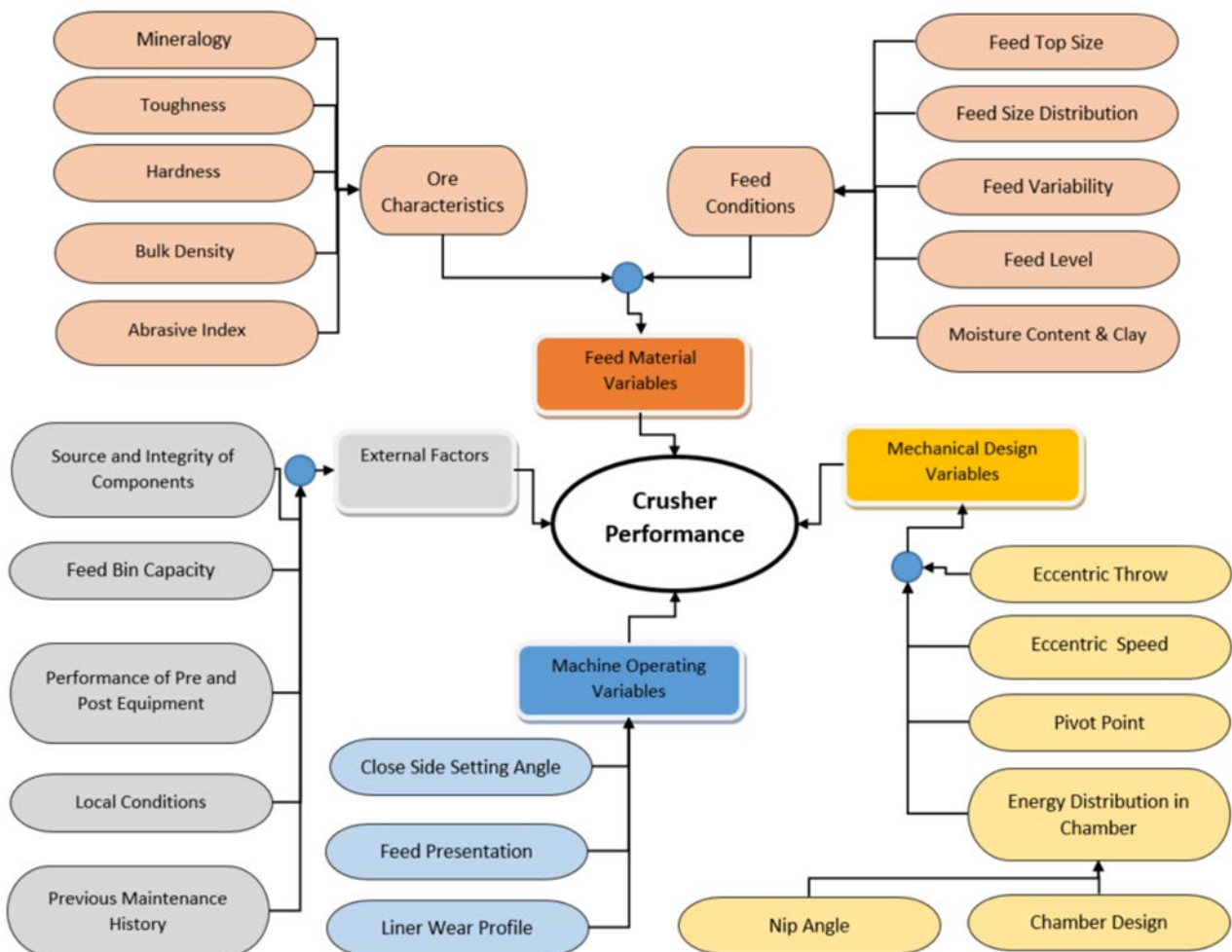
FIG 7 – Factors impacting crusher performance and liner wear (after Harding, 2018).
