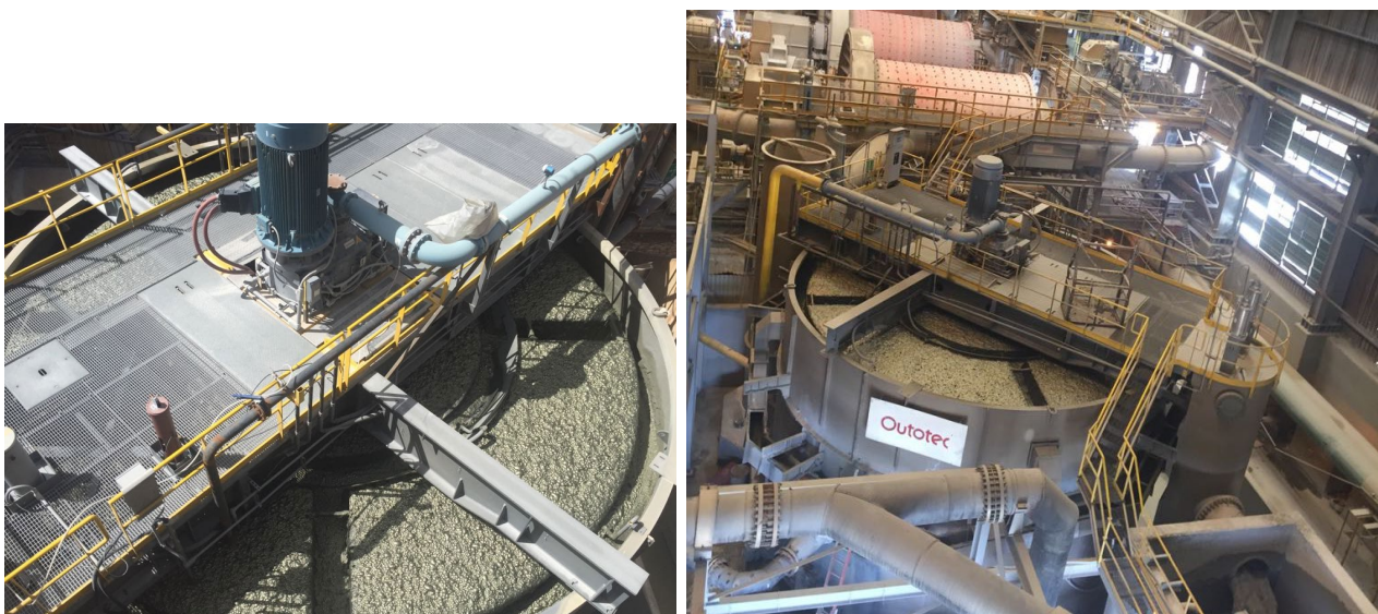
FIG 3 – TankCell® e630 flotation units: section 1 float cell to the right, installed outside the main concentrator building and section 2 float cell installed inside the main building.
