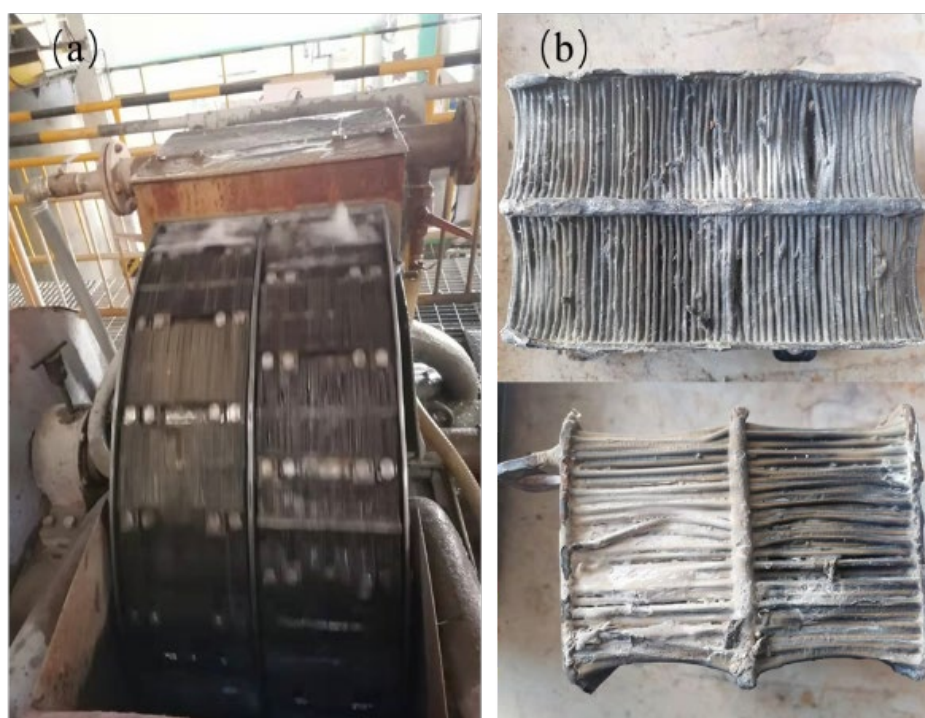
FIG 3 – The magnetic separator (a) and a fouled magnetic media pack (b).
