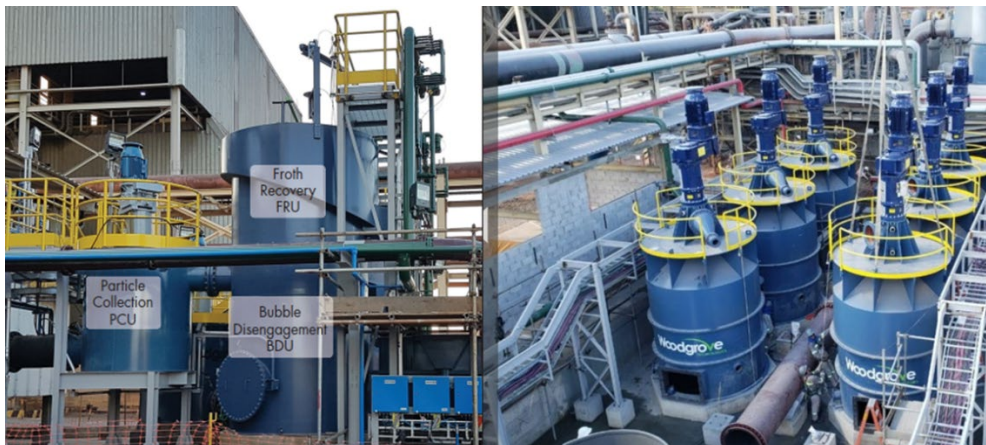
FIG 10 – Woodgrove Staged Flotation Reactor (left) and Direct Flotation Reactors (right) (Nelson and Lelinski, 2019; Woodgrove Technologies, 2022).
