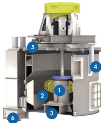
FIG 9 – Eriez StackCell®: 1. collection chamber, 2. separation chamber, 3. feed inlet, 4. froth, 5. wash water system, 6. tailings discharge (Eriez, 2022).
