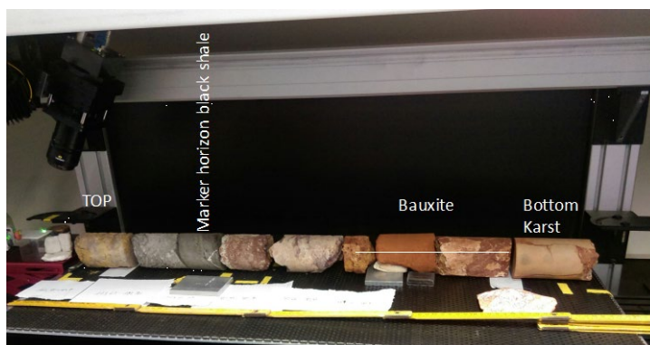
FIG 1 – LIBS measurement configuration of the composite bauxite profile for a line scan with the LTB core scanner from 2011 (from Meima et al , 2021).
