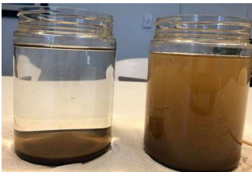
FIG 1 – Jar Test (0.6 ml/L on the left, Control on the right).
