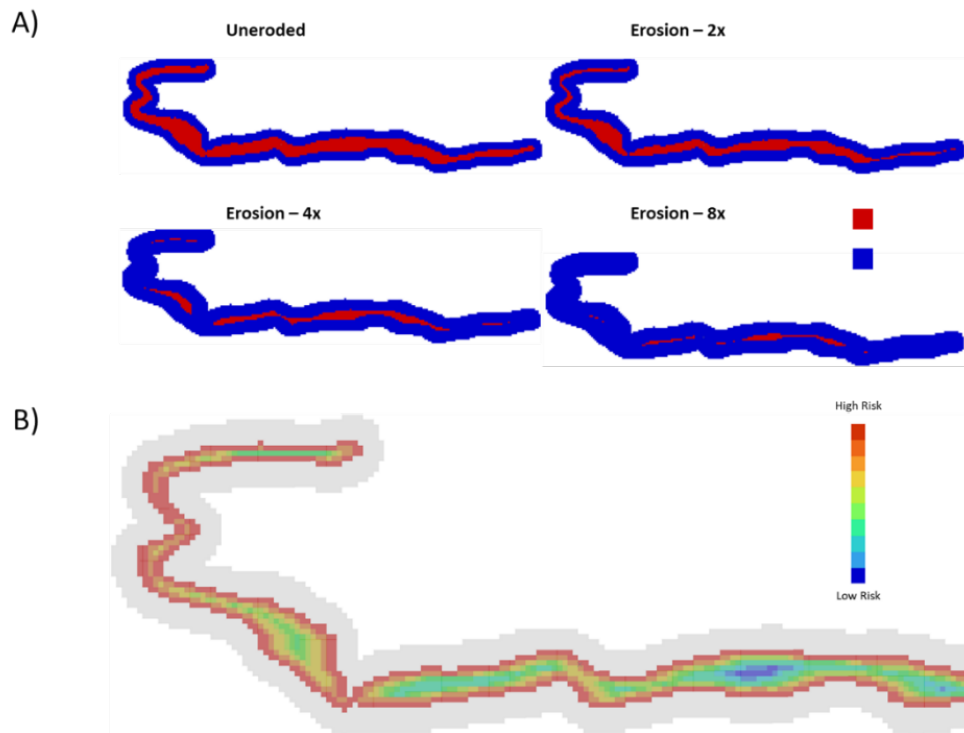
FIG 12 – (a) Mineralisation depletion from increased erosion; (b) risk map produced using the morphological operations approach.
