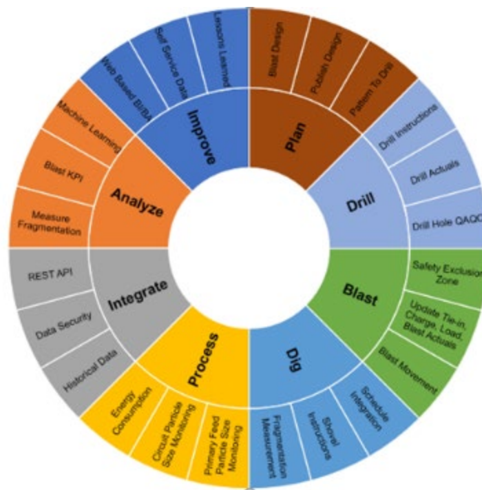
FIG 2 – Holistic drill and blast process.
