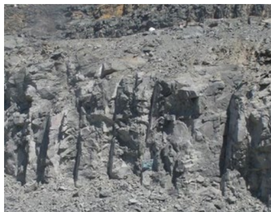
FIG 9 – Photo of saw tooth face profile in a southerly direction (Etchells, Sellers and Furtney, 2013).
