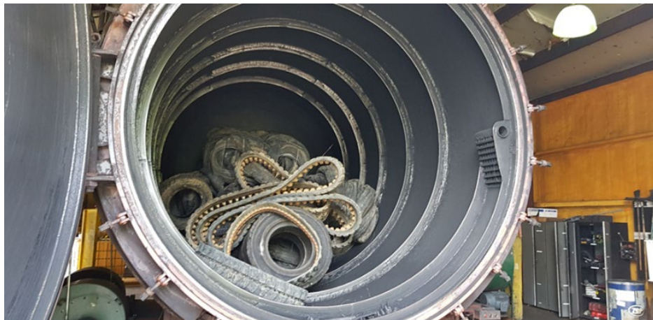
FIG 3 – Photo of the front-end of a GCI-103 reactor in Rome, GA, USA. Note the mixed waste rubber source.
