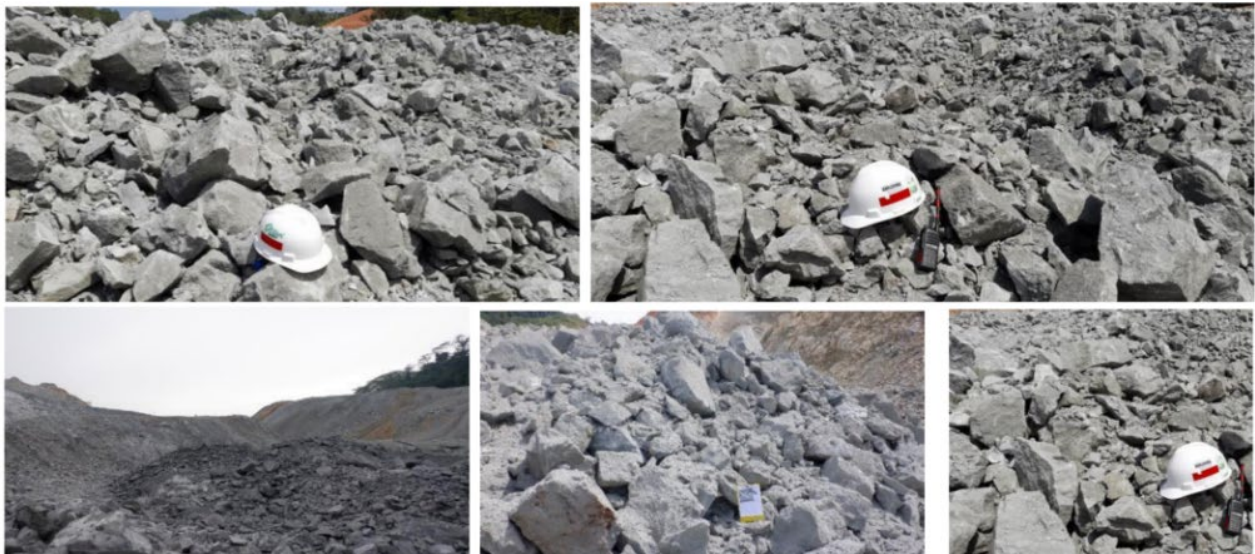
FIG 11 – Rock fragmentation by blasting.
