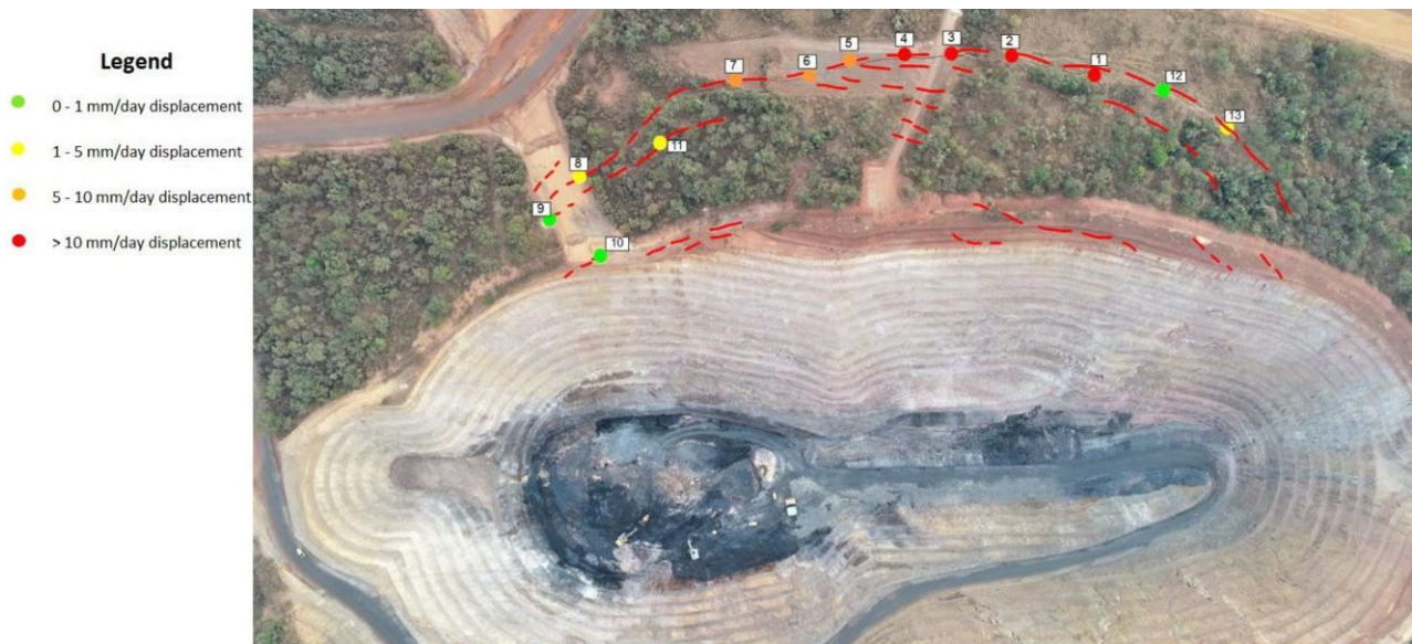
FIG 16 – Colour coded velocity plots of crack pins.
