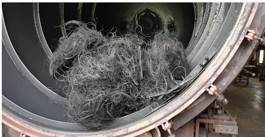
FIG 4 – Photo of the steel after the process had run its full course. Front-end of a GCI-103 reactor. Note the mixed steel in the reactor at the end of the process.
